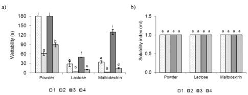
**Fig. 4.** Wettability (a) and solubility index (b) of infant milk powder before and after agglomeration; 15% lactose solution and 20% maltodextrin solution were used as wetting liquids The results are expressed as mean values with standard deviation. Values followed by a different letter are significantly different at p < 0.05.
